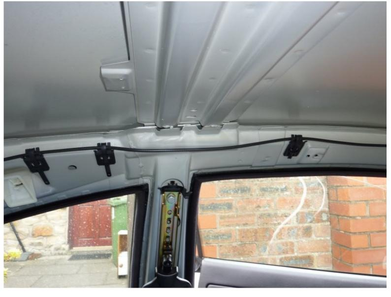
The rear covers do not need to be completely removed, just pulled away starting at the top and working down.
